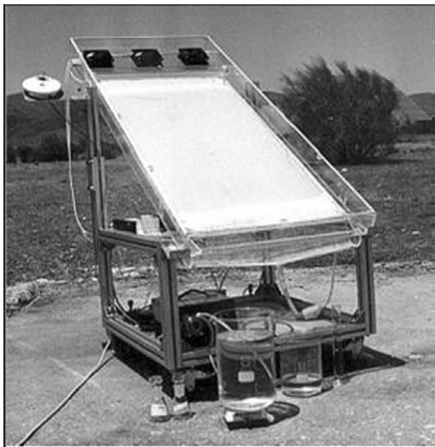
Figure 2 Thin film fixed bed reactor (reprinted from Bahnemann, 2004, with permission from Elsevier).
