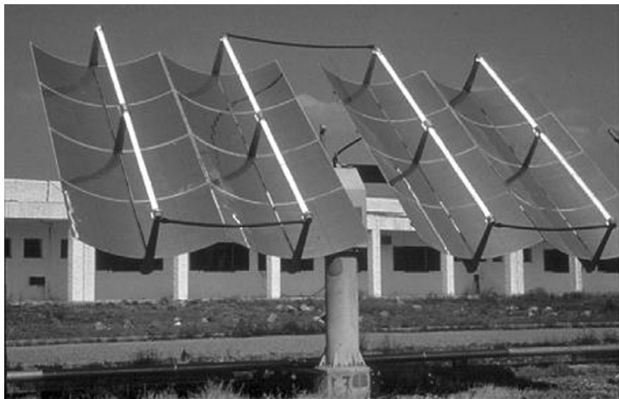
Figure 1 Parabolic trough photocatalytic reactor at Plataforma Solar de Almería (reprinted from Malato et al., 2007 with permission from Elsevier).
